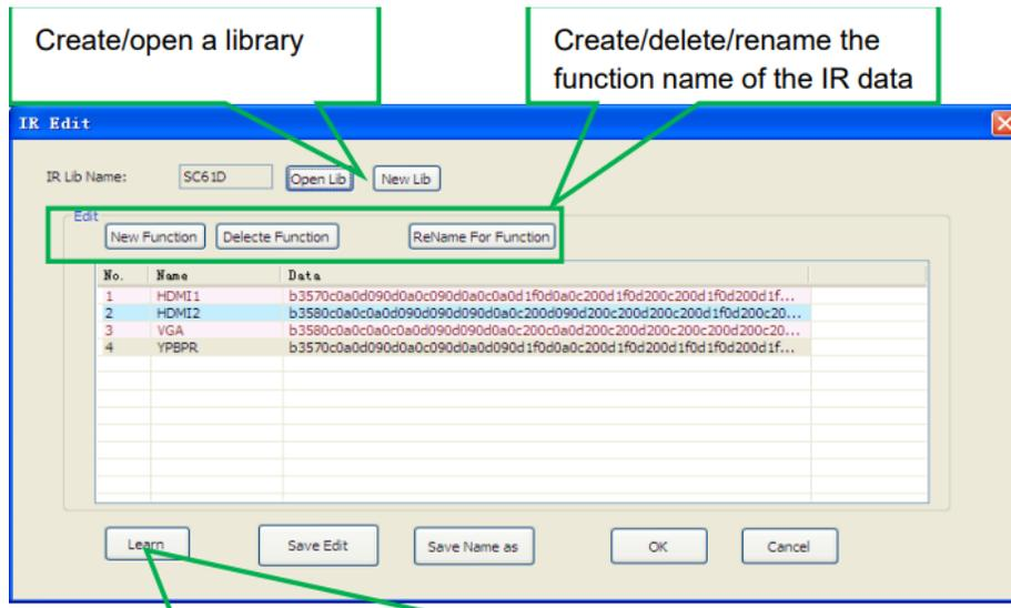
Select a function, and then click "learn", press the IR remote button to send the IR code to infrared sensor port, it will refresh the IR data. Follow the same steps can learn any function of the remote buttons.
