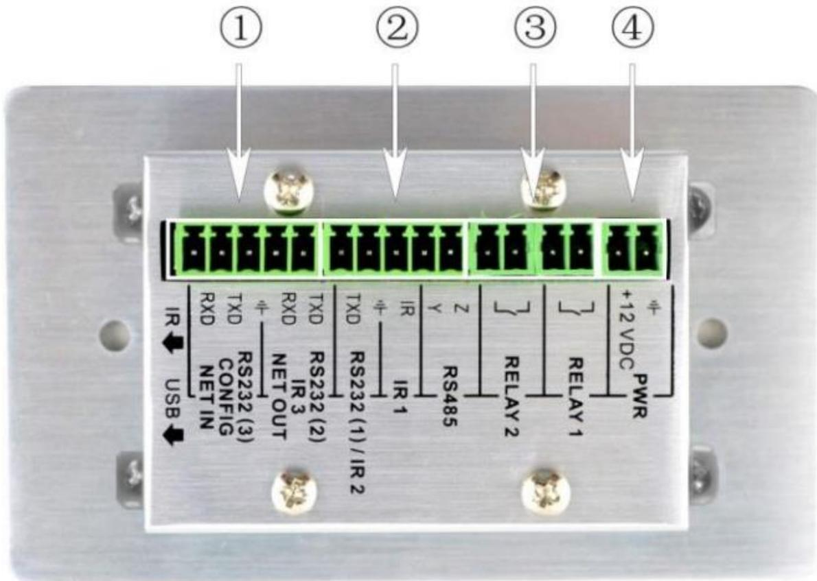
The programmable control panel has various ports in the rear panel, including Lopping port, RS232 port, RS485 port, IR port, Relay port and Power port. Below is the introduction:
