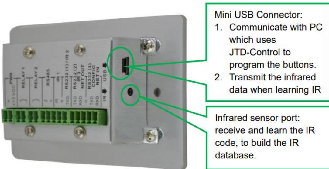
**Note:** When use this USB port to program the control panel's buttons, the available COM port number should not be more than 10.
