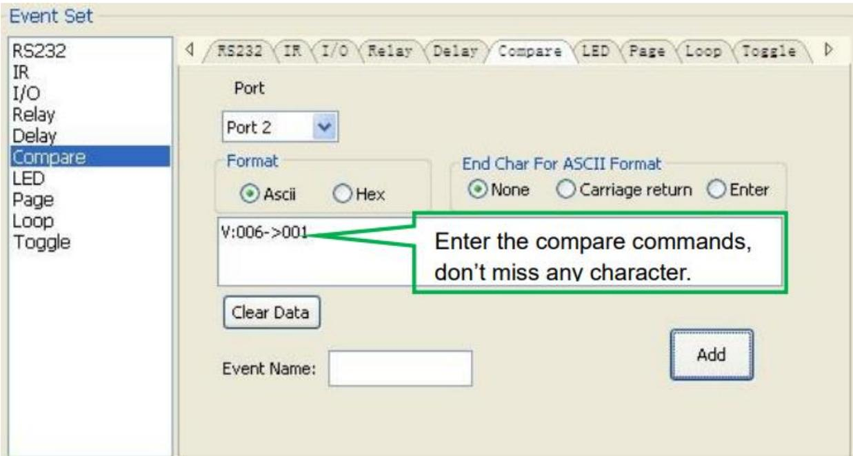
1. The send port must be selected as the same as model setting, otherwise the event cannot be added. And port 1 cannot be used for compare, for there is no a receive pin in this port.
