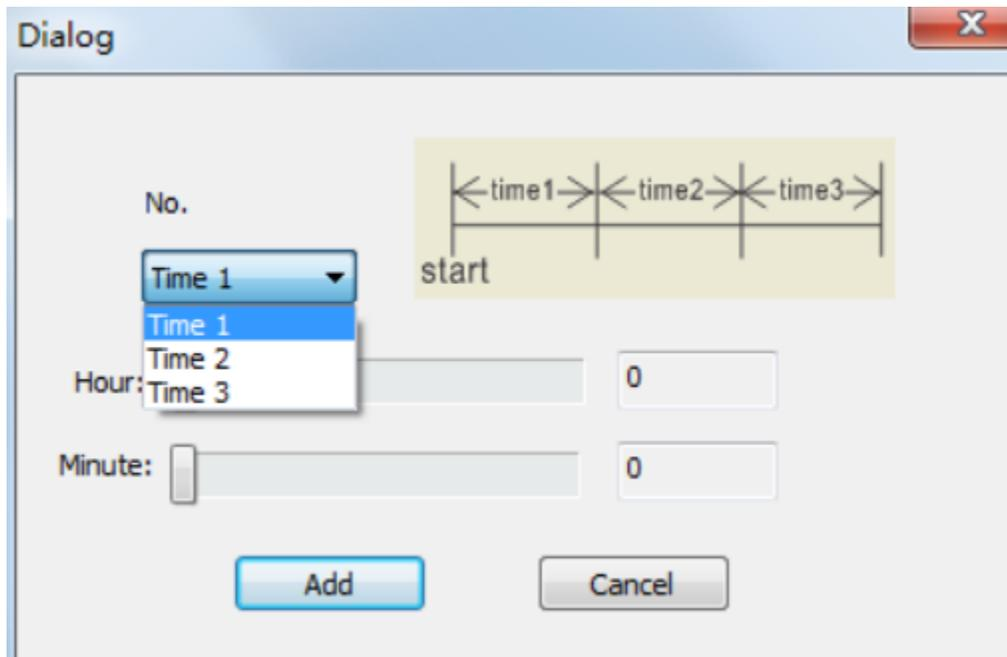
The time is counted from the programmable control panel start. When come to time1, the programmable control panel will execute the events in time1. Then recount from time2, and then time3.
