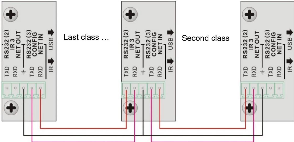
**Note:** Up to 99 programmable control panels can be looped within one system. However, to achieve normal interaction, loop less programmable control panels (10 tops) in the system
