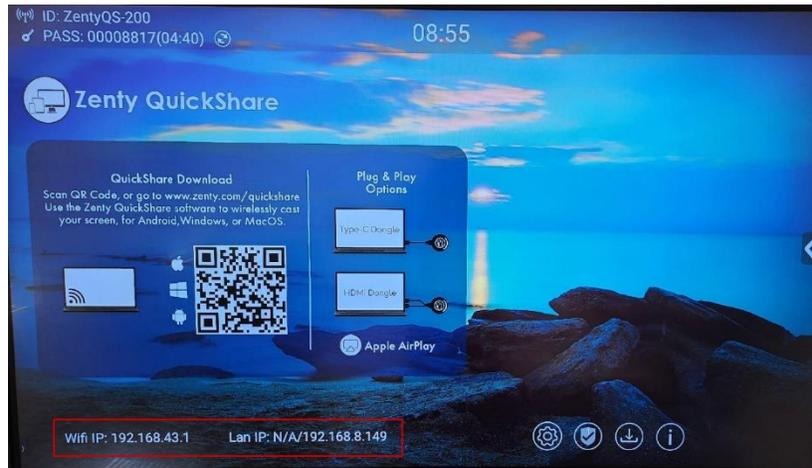
**Note:** When it shows “N/A”, means the ZT-QS200 is not connected to the LAN (Local Area Network) by CAT cable or it failed to get an available IP address by the corporation router.
